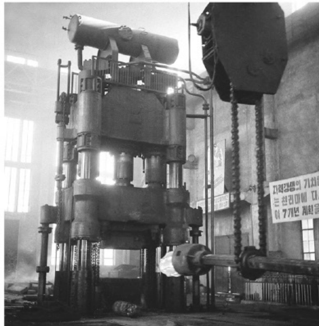
3 000-ton press manufactured by the Ryongsong Machine Plant
